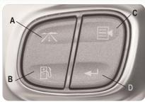
Trip Information: Press the Trip Information button (see "A" above) to display the odometer, two trip odometers and the trip timer. To reset the trip odometers or the timer to zero, press and hold the SELECT button (see "D" above) while the desired function is displayed. Use the SELECT button to start and stop the trip timer.
